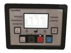
PowerStart 600 control operator /display panel
